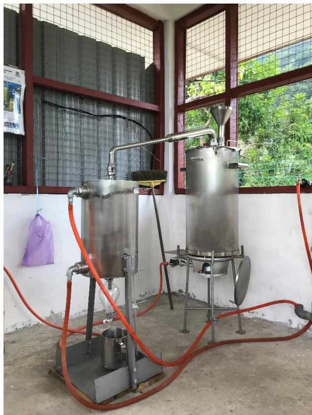
Figure 2: Distillation unit used to obtain Litsara essential oil
